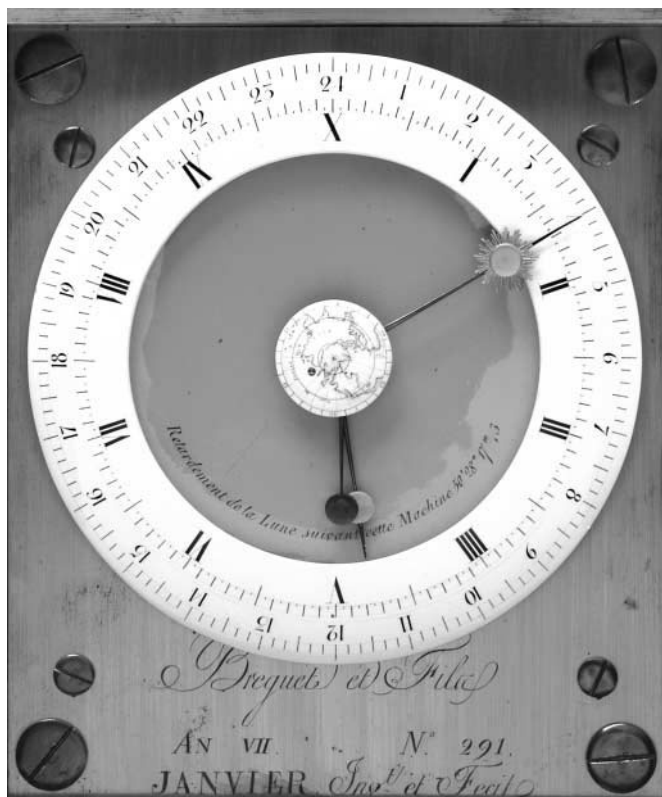
3. French revolutionary clockface, showing division into 24 hours (outer ring) and 10 hours (inner ring)
